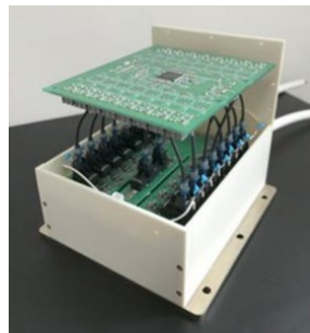
High-voltage switching modules
